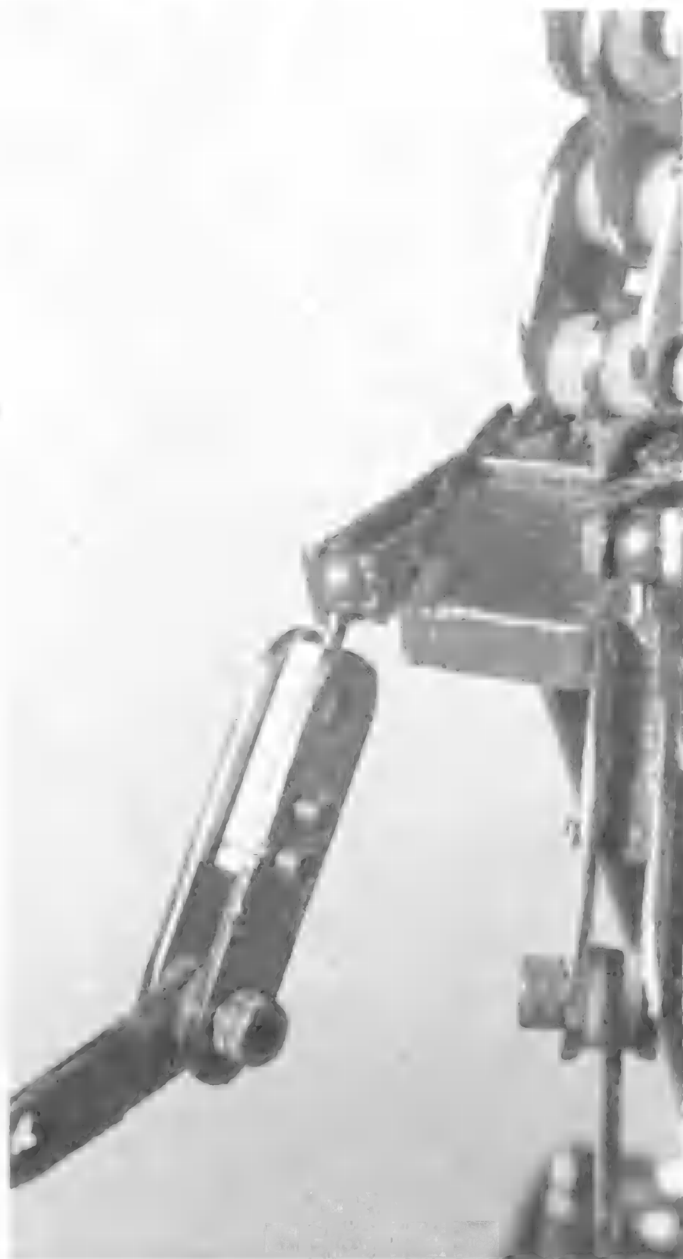
This ball joint is an aluminum ball sandwiched between two machined steel plates.
